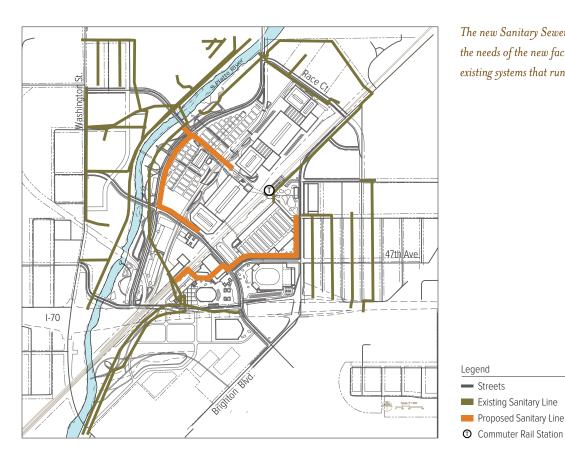
The new Sanitary Sewer System will address the needs of the new facilities and tie into the existing systems that run along the river.
